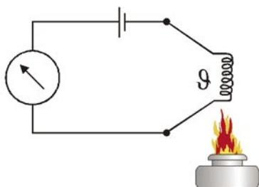
Resistance temperature devices capitalize on the fact that the electrical resistance of a material changes as its temperature changes. As their name indicates, RTD's rely on resistance changes in a metal, with the resistance rising more or less linear with temperature.
