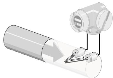
The DMU Prosonic Flow sensors (clamp on version) are mounted directly onto existing piping. Isolating or opening the piping is not required. The system is ideal for bidirectional measurement of pure or slightly dirty liquids. The Prosonic Flow is especially suitable when retrofitting equipment as no interruption of the process is necessary.
