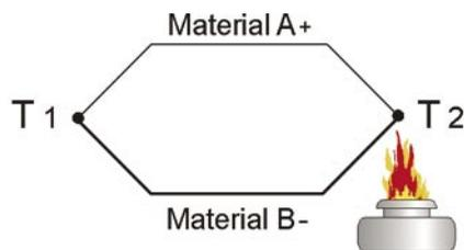
When two wires composed of dissimilar metals are joined at both ends and one of the ends is heated, there is a continuous current which flows in the thermoelectric circuit.
