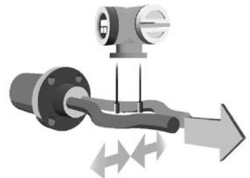
The Promass I has a full bore, straight-through, single-tube design which operates somewhat differently than the dual-tube design. In order to maintain balance for flawless measurement, a patented Torsion Mode Balanced (TMB) system is used. By exciting an eccentrically located, counter-oscillating pendulum mass, the single tube system provides accurate measurement, even with changing process and ambient conditions.
